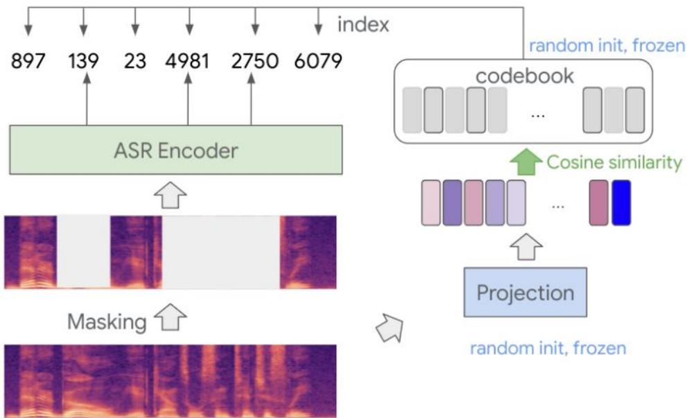
Figure 3: BEST-RQ based pre-training with conformer encoder.
